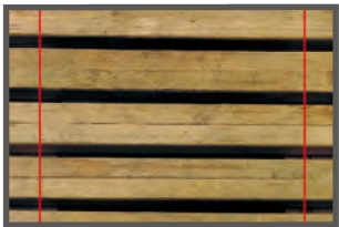
雷射顯示紙張位置 Laser indicator to pre-display the paper location
