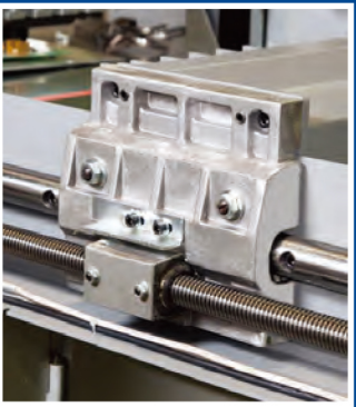
高精密密度螺桿與雙導軌 Ball screw for high precision cut
