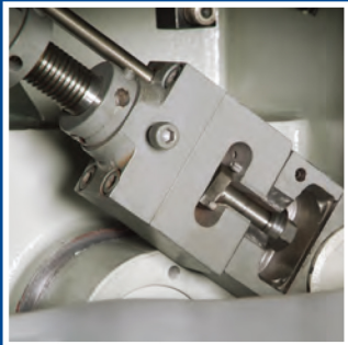
刀調整及拉刀臂保險螺絲 Device for Safety and easy Blade Adjustment procedures
